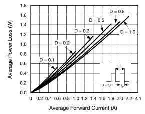
Fig. 2 - Average Power Loss Characteristics
