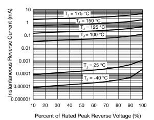
Fig. 4 - Typical Reverse Leakage Characteristics
