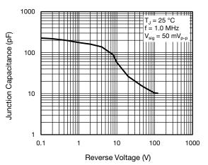
Fig. 5 - Typical Junction Capacitance
