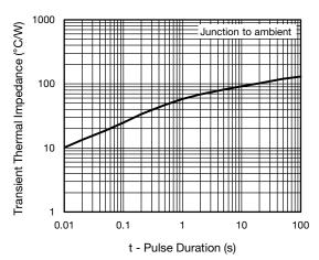
Fig. 6 - Typical Transient Thermal Impedance
