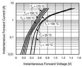
Fig. 3 - Typical Instantaneous Forward Characteristics
